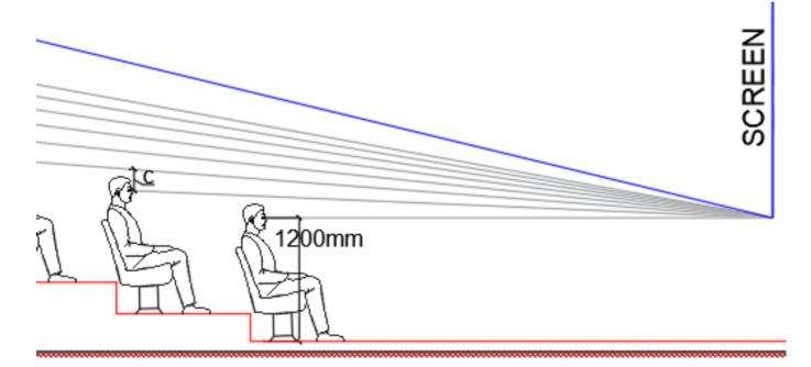
If all risers have equal heights, the sightline clearance decreases with increasing distance from the screen. To get acceptable sightline from the last rows, the risers might be very high, and the total height of the stadium will be very big. That will again lead to larger projection angle and increased image distortion (keystone). The sound reproduction will also suffer.
